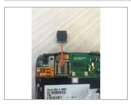
To install the new camera sensor, place in slot. Reassemble phone by doing steps 1-3 in reverse order.
