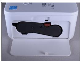
Open the door to the ink cartridge located on the right-hand side of the printer.
