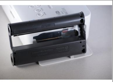
Pull out the empty ink cartridge and exchange it with a new one.
