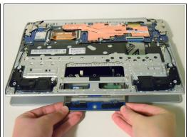
With the laptop slightly open, push the trackpad upwards at the rear, and pull it out from the bottom.
