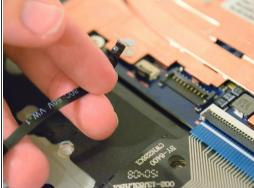
Remove the connector between the trackpad and the motherboard by pulling upwards on it at the port.
