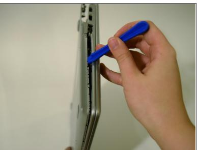
Loosen the back cover panel with a plastic opening tool, and work it all the way around the computer.
