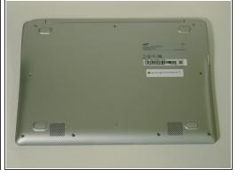
Remove the nine 5 mm screws on the bottom cover using a Phillips #0 screwdriver.
