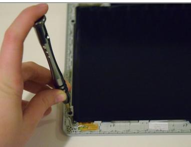
Using a Phillips #0 screwdriver to unscrew the four 3 mm screws keeping the screen in place.
