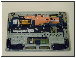
• Disconnect the wire that connects the battery to the motherboard by pulling upward.
