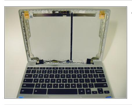
Pull the screen from the front panel using your hands to fully remove it.
