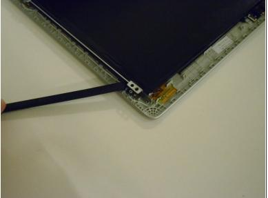
• Using the spudger, pry the screen loose from the front panel.
