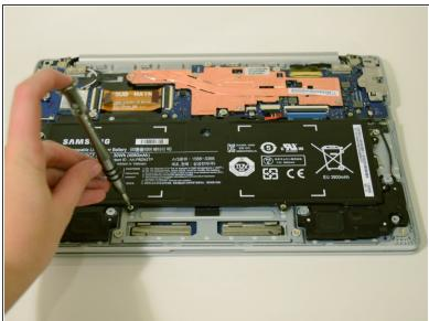
Unscrew the four 4 mm screws holding the battery in place with a Phillips #0 screwdriver.
