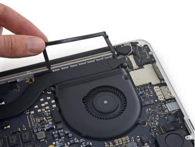
• Peel the left rubber cover up off the fan and fold it out of the way.
