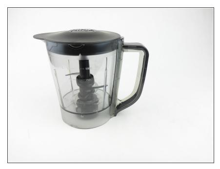
Begin by removing the blender from the base. This requires only a twist counterclockwise and a pull up.
