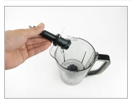
Remove the lid and and pull straight up on the blender blade. It will come out easily.
