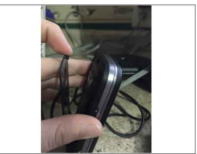
Simply push the button on the top and pry (with hands) the back cover off.
