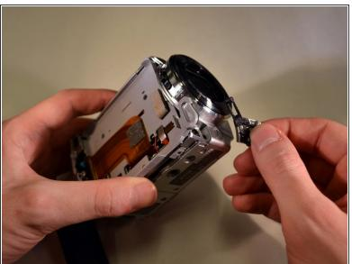
Using your fingers, remove the A/V tab.
