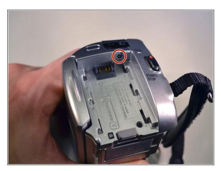
On the back of the device, unscrew the top 3mm Philips screw.
