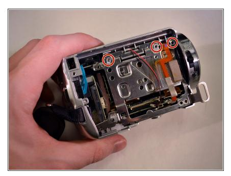
Unscrew the top 3 3mm Philips screws from right to left.
