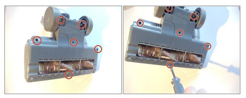
• Carefully unscrew the 6 screws with a Phillips screwdriver. Set aside.
