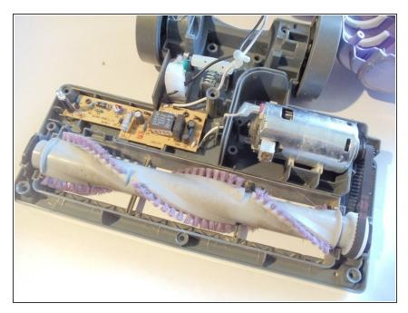
• Return the clean brush roll and resituate the belt to secure it in place.
