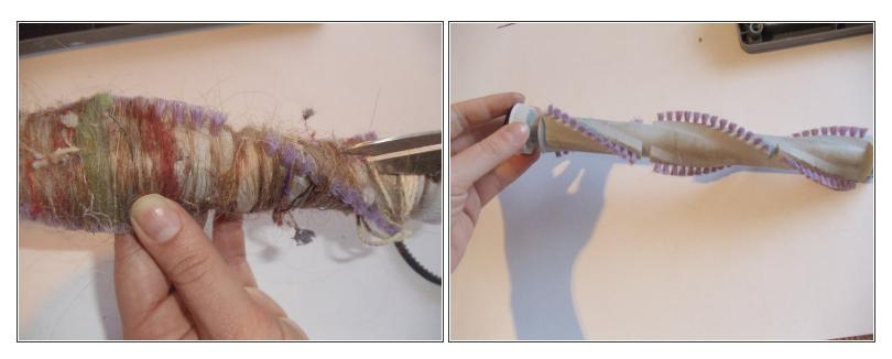
• Use scissors to cut strings and other debris from the brush roll. Avoid cutting the bristles.
