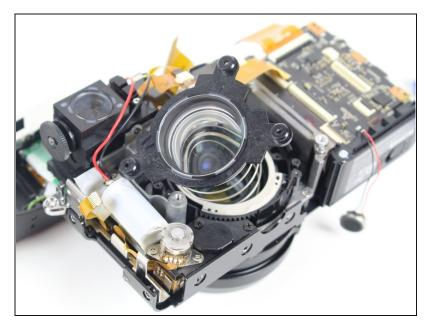
• Remove the spring and the lens by gently lifting both the components upwards.
