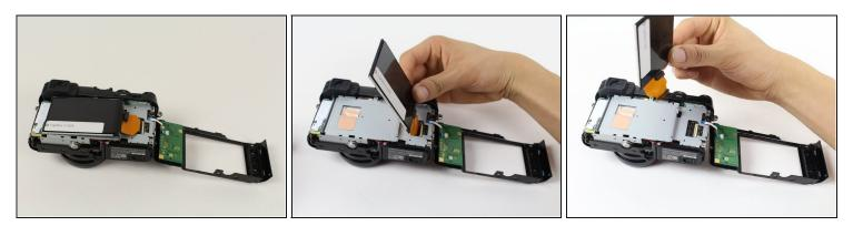
• Remove the orange ribbon cable by opening up the ZIF connector with a plastic prying tool or toothpick.
