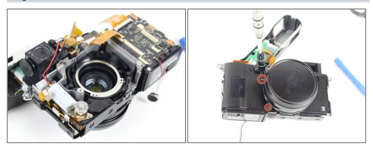
• Once the lens has been taken off, flip the camera over and unscrew the two 4.0 mm screws on the front of the camera, next to the lens cover.
