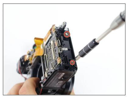
Remove the two 4.0 mm screws located on the side of the camera.
