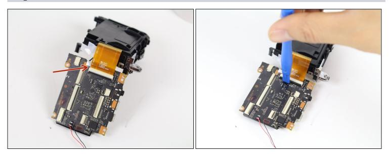
• Use the plastic opening tool to remove the orange ribbon on the motherboard by wedging the tool under the ribbons black tab, and carefully prying upwards.
