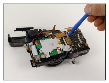
• Use a plastic opening tool to pry off the ribbon located next to the top-right of the green sensor board.
