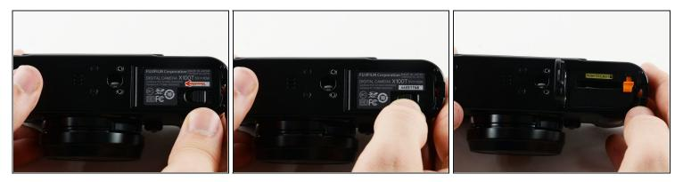
• Slide the small black tab on the bottom of the camera to the left to unlock the battery cover.
