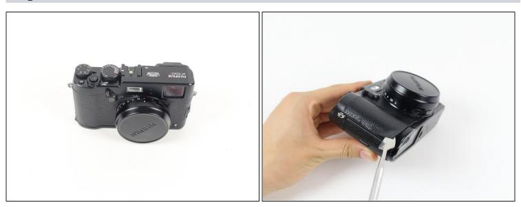
• Beginning in one of the corners, use a spudger to pry the leather casing off of the camera.
