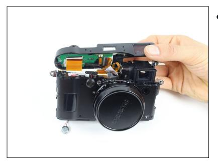
• Remove the top frame by lifting it off and pulling it towards the backside of the camera.
