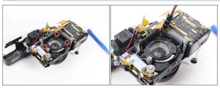
• Remove the three 3.5 mm screws on the spring-loaded cover.
