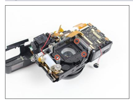
• Remove the three 3.5 mm screws on the black lens cover.
