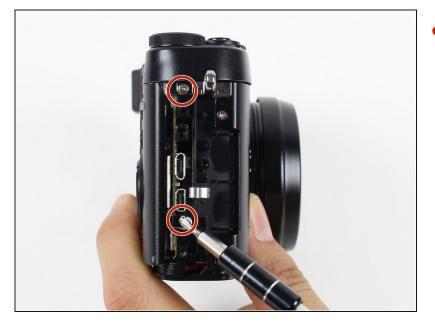
Remove the two 6.0 mm screws beneath the port cover assembly.
