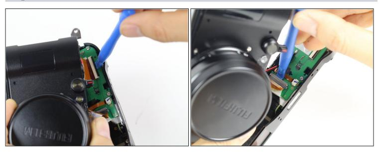
• Use a plastic opening tool to detach the two ribbon cables from the top frame.
