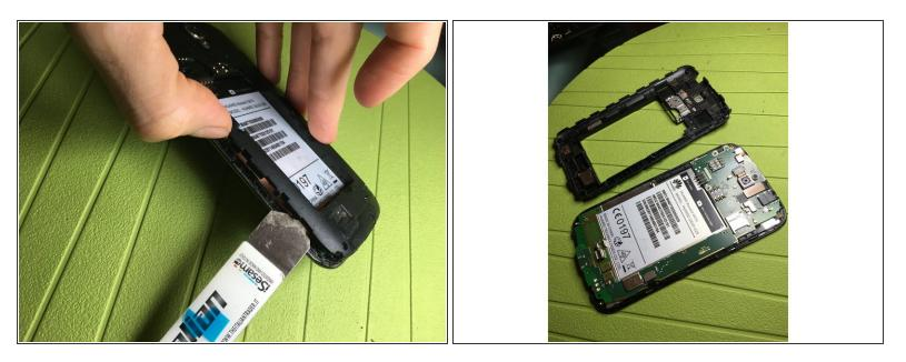
• With the help of a thin tool, pry laterally on the joints and remove the central body
