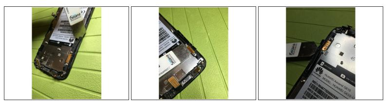
• With the help of a heat source, remove the audio and power button ribbon cable
