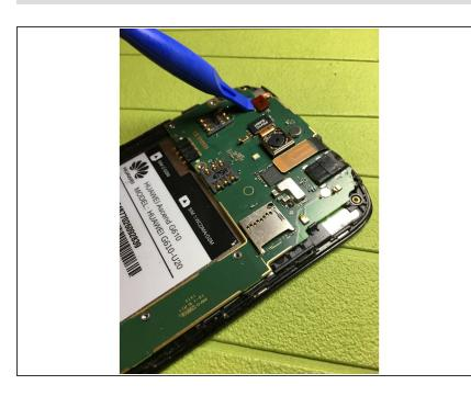
• Disconnect the light sensor connector.
