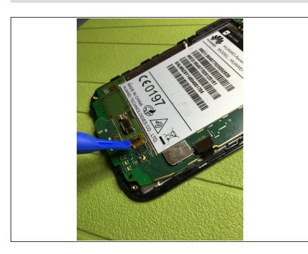
Pry out the connector between the two boards
