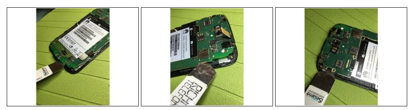
• With a thin tool, help us to unhook the motherboard from the joints
