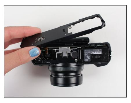
Carefully lift up the bottom piece of the camera to remove it.
