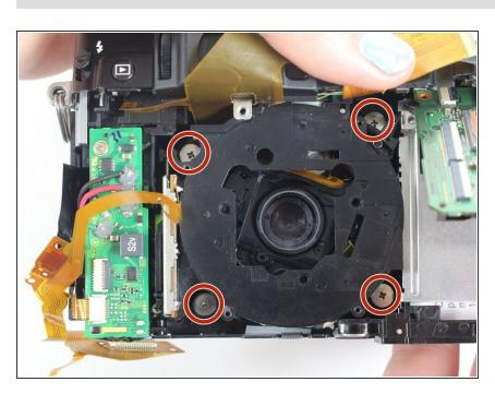
Remove the four 4.4 mm silver screws at the corners of the lens using a Phillips #000 screwdriver.
