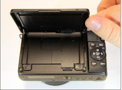
Rotate the LCD screen away from the camera.
