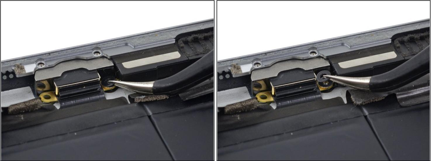
ⓘ The screw through the Lightning connector has a small washer resting on the speaker contacts. Be sure not to misplace it.
