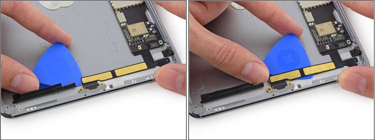
ⓘ The Lightning connector cable is stuck to the case with some adhesive. To detach the adhesive you will be sliding an opening pick between the cable and the case. Be very careful not to cut the Lightning connector cable itself.
