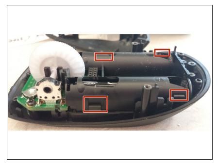
4x plastic clips hold the battery case. To remove, un-clip one side and tip out.
