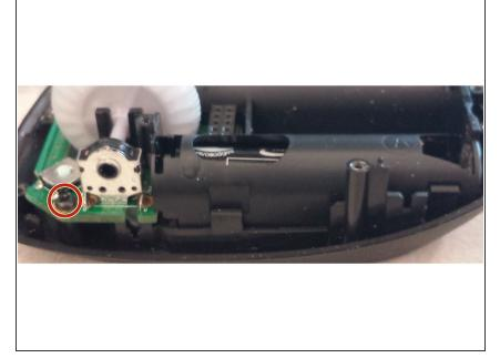
2x phillips 00 screws hold the wheel and button assembly. I never removed this because of the two buttons underneath. Any further tear down should be simple.
