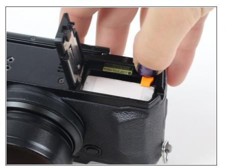
Once you have the battery compartment open, slide the orange tab away from the battery until it ejects.
