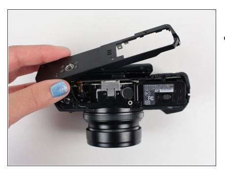
Carefully remove the bottom piece of the camera.
