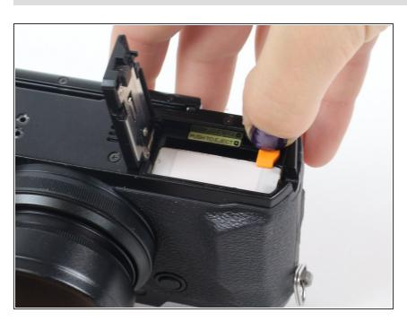
Once you have the battery compartment open, slide the orange tab away from the battery until it ejects.
