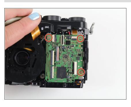
Remove the three 2.6 mm screws located in the top two corners and the bottom right corner of the motherboard using a Phillips #000 screwdriver.
