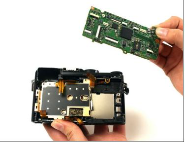
Start at the top of the camera and use the plastic spudger to pry the motherboard out of the camera.
