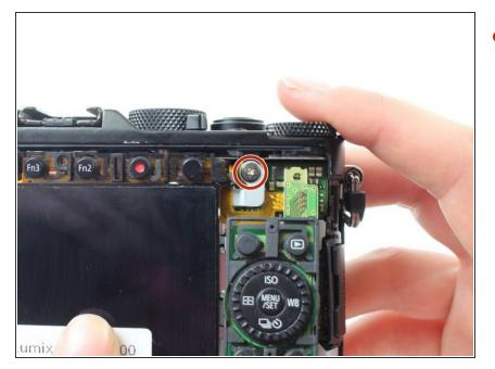
Use a Phillips #000 screwdriver to remove the 7.5mm screw on the top right of the back of the camera that holds the metal backing in place.
