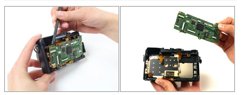
Start at the top of the camera and use the plastic spudger to pry the motherboard out of the camera.
