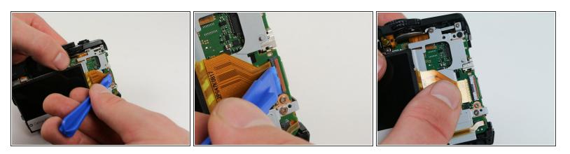
A Do not pull the connector upwards as doing so may harm the connector housing.
