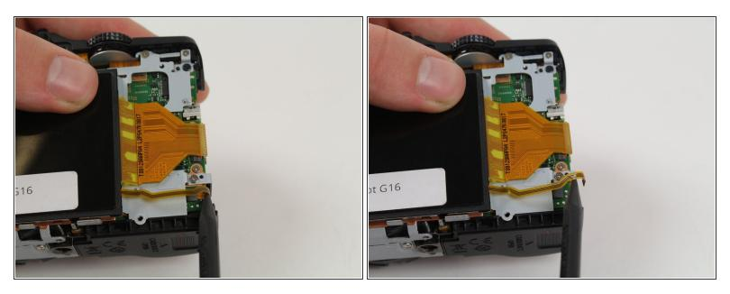
Unplug the small connector ribbon by pulling the cable outwards from the camera using a spudger or your fingers.
