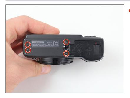
• Remove the four 3.3 mm screws on the bottom of the camera using a Phillips #00 screwdriver.
