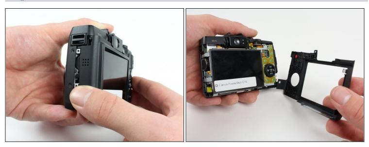
• Using your fingers, carefully pull the the back cover off by grabbing the bottom left of the back cover and pulling outwards.
