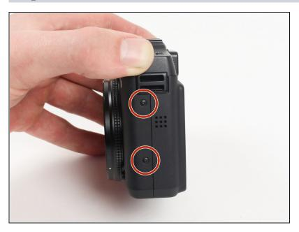
Remove the two 3.3 mm screws near the speaker using a Phillips #00 screwdriver.
