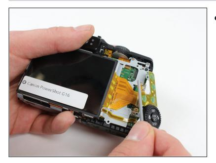
• Lift the button circuit board away from the camera.
