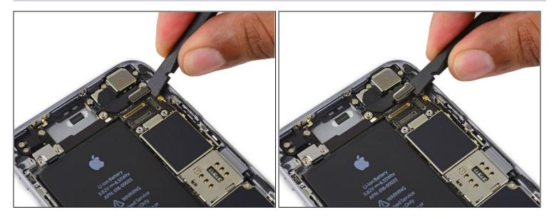
• Use the flat end of a spudger to disconnect the rear camera from its socket on the logic board.
