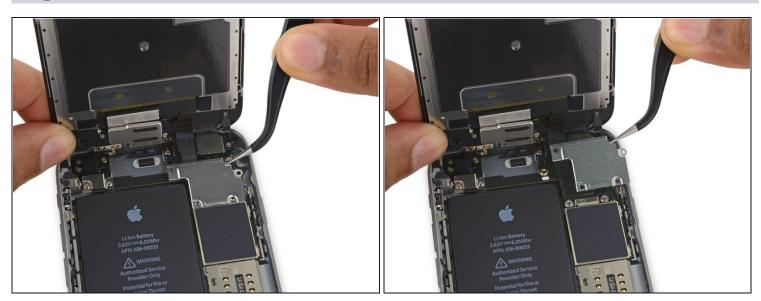
• Remove the display cable bracket.
