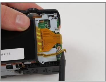
• Unplug the small connector ribbon by pulling the cable outwards from the camera using a spudger or your fingers.
