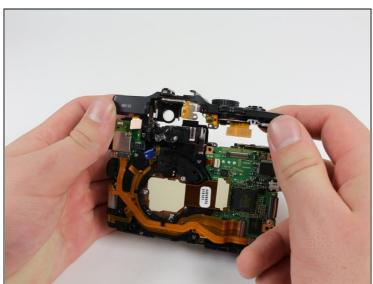
• Remove the top portion of the casing by firmly grasping it and pulling it upward to lift it off.
