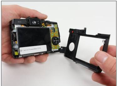
• Using your fingers, carefully pull the the back cover off by grabbing the bottom left of the back cover and pulling outwards.
