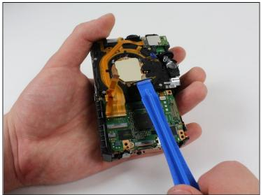
Disconnect the lens cable from the motherboard by lifting it up vertically from the motherboard using a plastic opening tool.
