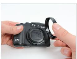
• Remove the ring around the lens by simultaneously pressing the black button located at the bottom right of the ring and rotating the ring counterclockwise.
