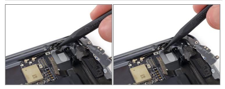
• Use the tip of a spudger to pry the small metal retaining clip off the antenna cable.
