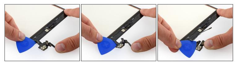
• Use an opening pick to break up the adhesive holding the home button ribbon cable to the digitizer cable.
