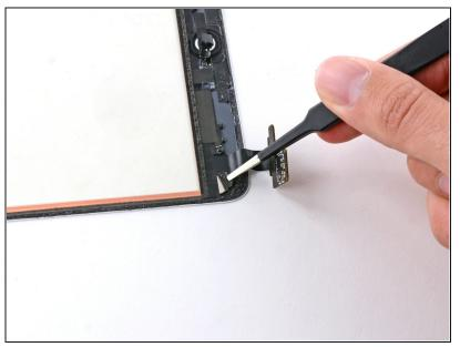
(i) If necessary, use a pair of <u>tweezers</u> to partially peel back the piece of tape covering the smart cover magnet near the lower left corner of the front panel assembly.
