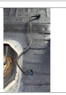
• with the access panel now removed, you're ready to start removing and replacing the pipes. I started with the outlet which is the bigger of the 2 and the one closest to the rear of the vehicle. Just press both sides of the quick connect coupling in simultaneously and pull it off. Then go underneath and remove it from there.
