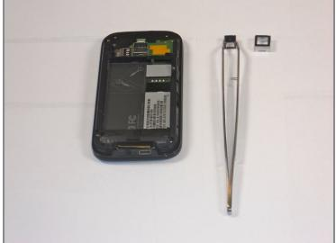
• Use the <u>tweezers</u> to pull the camera cover up and away from the phone. Repeat for the camera underneath.
