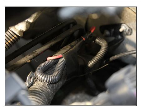
Identify the auxiliary wire, which is folded and taped to either the wiring harness or the fire wall.
