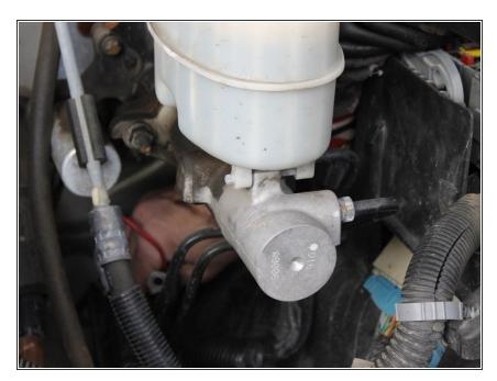
Locate the wiring harness bundle, which exits the firewall underneath the brake booster.
