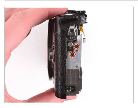
Use a Phillips #00 screwdriver to remove the two 1.6 mm screws near the left hand grip.
