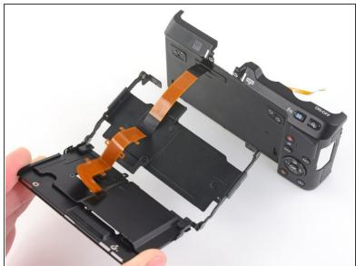
Pull the LCD assembly away from the back case.
