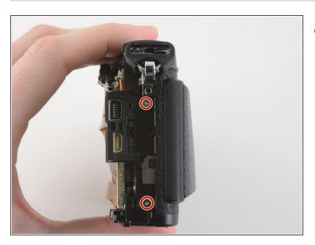
Remove the two 4.1 mm Phillips screws near the right hand grip.
