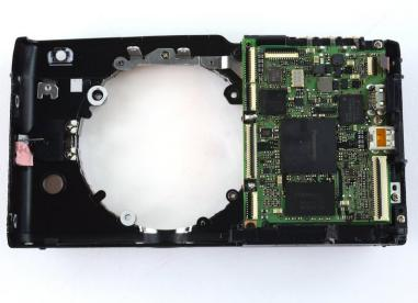
Remove the sensor assembly from the front case.
