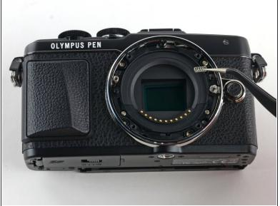
• Use tweezers to remove the two springs lying beneath the inner metal ring.
