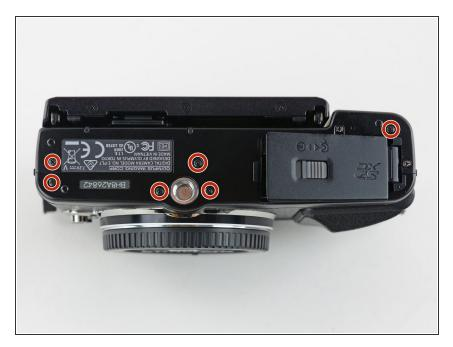
Use a Phillips #00 screwdriver to remove the six 2 mm screws on the bottom of the camera.
