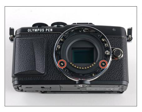
Remove the two 4 mm Phillips screws.
