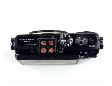
Use a Phillips #00 screwdriver to remove the four 4 mm screws from the external flash port.
