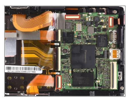
Use a spudger to remove the three indicated ribbon cables from their ZIF connectors on the motherboard.
