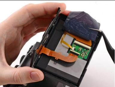
Use tweezers to remove the plastic covering the LCD ribbon cable.
