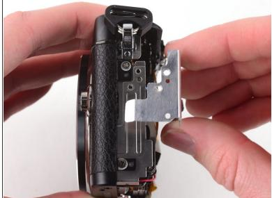
Once the screws are removed, use two fingers to remove the metal clip.
