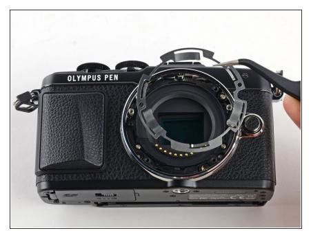
Use tweezers to remove the inner metal ring.
