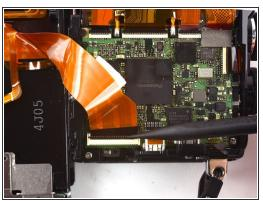
To remove the ribbon holding the back case to the camera, use the pointed end of a spudger to flip back the top bar on top of the ZIF connector.
