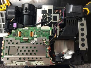
Disconnect the ribbon cable connected to the LEDs on the outside of the case.
