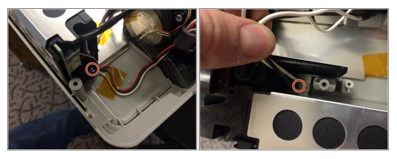
Remove the 2 screws from the front and back of the lamp ballast holder.
