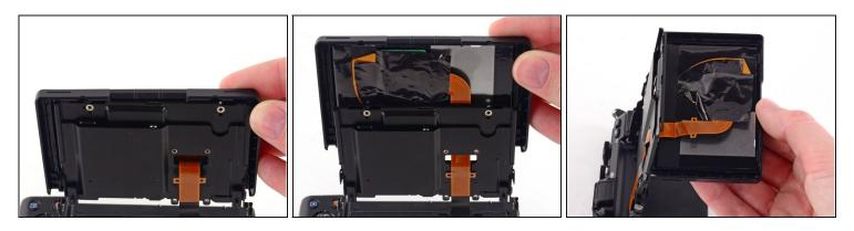
• Carefully lift the LCD screen up and away from the assembly.
