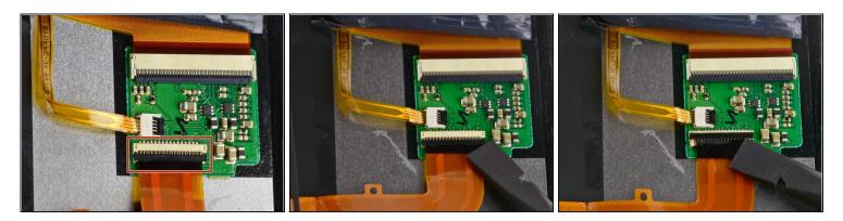
Use a spudger to flip back the black bar on the LCD Ribbon ZIF connector.
