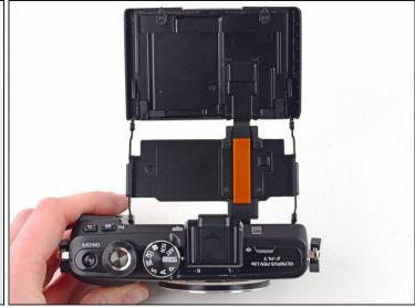
• Fully extend the LCD assembly.
