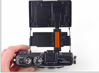
Fully extend the LCD assembly.
