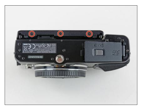
Use a Phillips #00 screwdriver to remove the three 2.3 mm screws from the base of the LCD screen.
