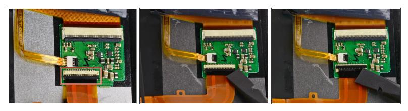
Use a spudger to flip back the black bar on the LCD Ribbon ZIF connector.
