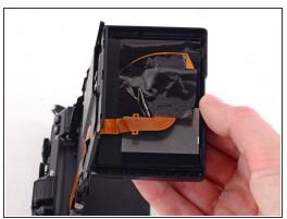
Carefully lift the LCD screen up and away from the assembly.
