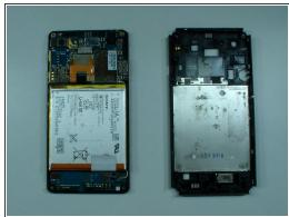
• Use a plastic tool and separate the rear bezel.
