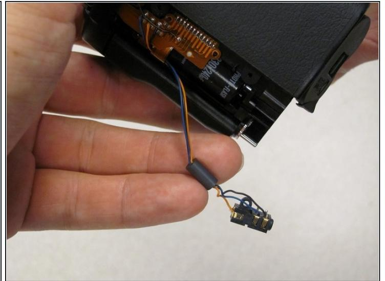
ⓘ The control socket is now secure by three wires.
