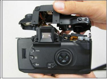
• Slowly separate the top panel from the camera by pushing it upward.
