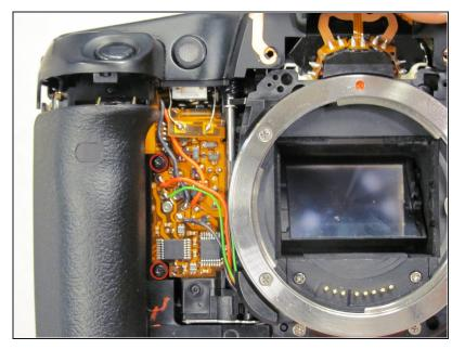
• Remove the two 5.5 mm screws from front of camera.
