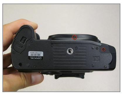
Remove the 4.3 mm black screw under the lens ring, and the 4.8 mm black screw under the camera.
