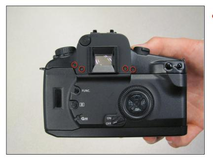
Remove the four 4.3 mm black screws near the bottom corners of the eyepiece at the back of the camera.
