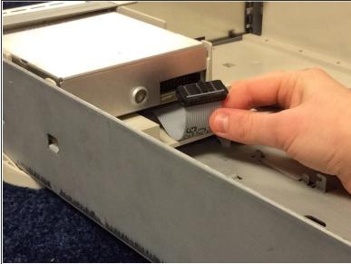
Disconnect the floppy cable from the drive, pulling on the cable.
