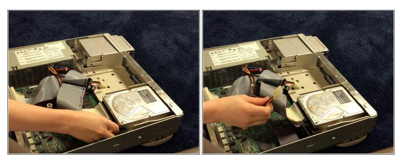
Grab the power connector for the hard drive and take it out of the hard drive.
