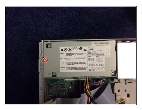
Unscrew the screw holding the power supply in place with the #1 Phillips screwdriver.
