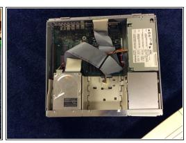
To start, lift the two tabs on the back of the computer and take the cover off.
