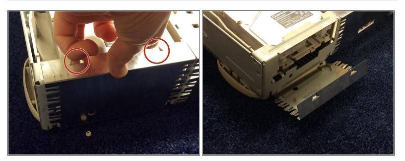
Push up on the two tabs for the EMI shield, and fold it down.
