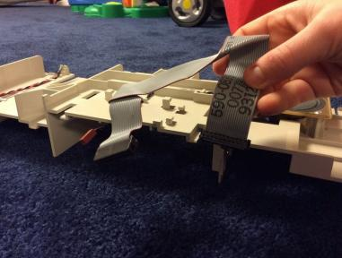
Flip the internal chassis over, and take out the floppy cable, carefully unthreading it from its routing guides.
