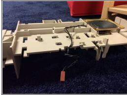
Carefully remove the speaker wire from its routing guides.
