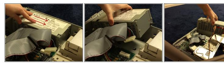
Push the power supply toward the front of the computer, lift up the side of the power supply closest to the floppy drive, and take the power supply out of the Mac.
