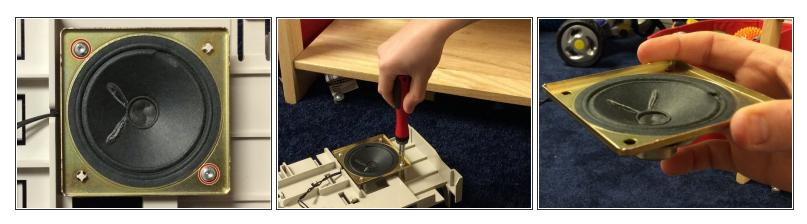
Unscrew the two marked Torx screws with your <u>T10 Torx screwdriver</u> and remove the speaker.
