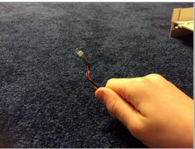
Take out the LED cable, carefully removing it from its routing guides.
