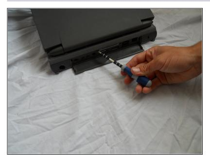
• Open the panel on back of the device. Remove 2 T8 torque screws.
