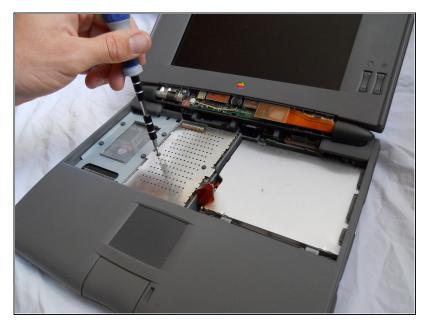
Remove the 2 T8 Torx Screws securing the logic board protection plate from the midsection of the logic board protection plate. Remove the T8 Torx Screw from the back of the plate, underneath the hinge.
