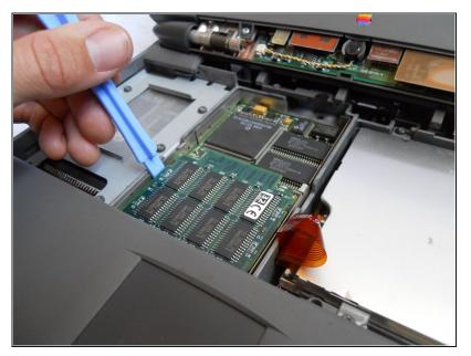
• Using a plastic spudger, gently pry up the uppermost board fixture. This is the Memory (RAM).
