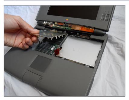
• Remove the logic board protection plate.
