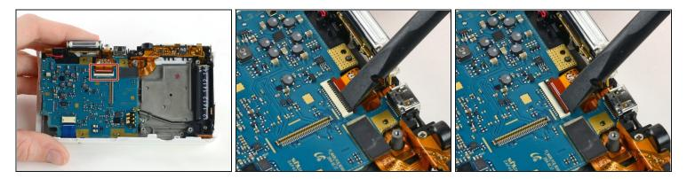
• Use a spudger to unlock the topmost ZIF connector by flipping open the black flap.
