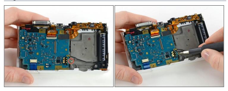
• Use a Phillips #00 screwdriver to remove the 3 mm screw located below the wifi antenna.
