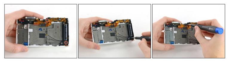
• Use a Phillips #00 screwdriver to remove the two 5 mm screws holding the flash assembly to the camera case.
