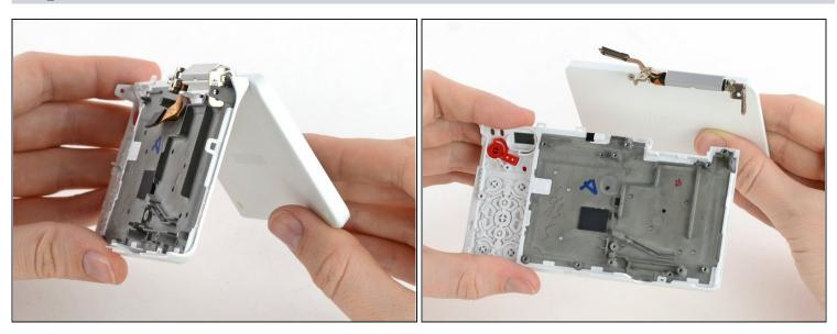
• Tilt and wiggle the LCD to remove it from the case.
