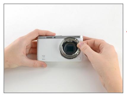
• Remove the metal lens mount by hand or with <u>tweezers</u>.
