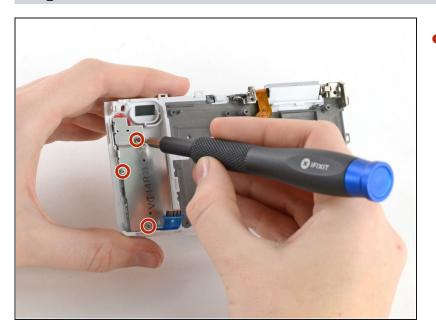
• Remove the three 4 mm Phillips #00 screws securing the button panel to the camera case.
