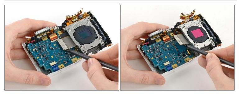
• Use a spudger to disconnect the ribbon cable connecting the image sensor to the motherboard.
