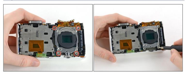
• Remove the four 4 mm Phillips #00 screws holding the sensor mount in place.
