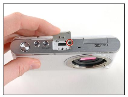
• Remove the 4 mm Phillips #00 screw hiding in the external flash port.
