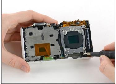
• Remove the four 4 mm Phillips #00 screws holding the sensor mount in place.
