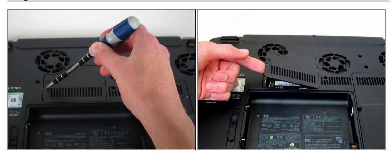
• Loosen the Phillips screw labeled 'ram' and lift the cover.
