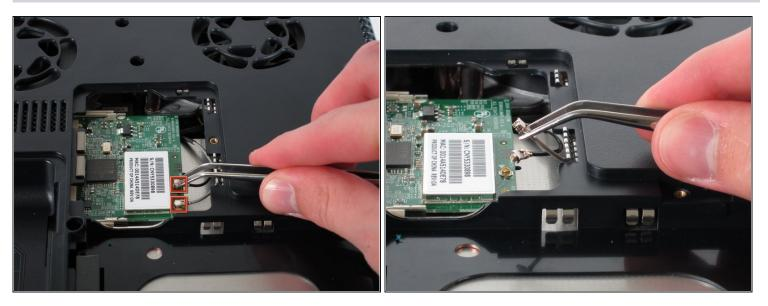
• Use <u>tweezers</u> to detach the grey and black cables connected to the green WiFi card.
