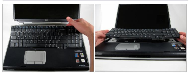
$\triangle$  Lift the keyboard carefully because it is attached to the motherboard by a ribbon cable.
