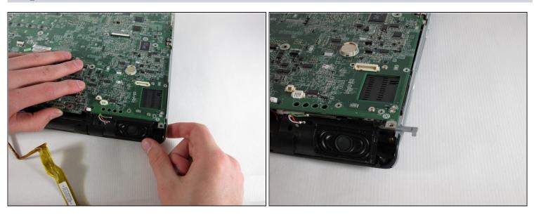
• Turn the computer 90 degrees counter-clockwise and clear all cables off of the motherboard.
