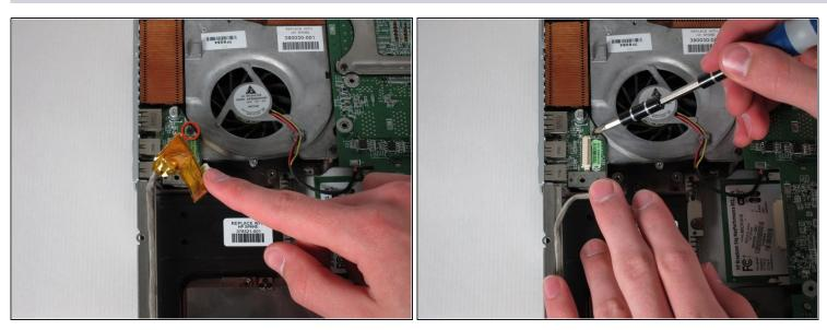
• Unscrew the 6mm Philips screw connecting the USB module to the fan.
