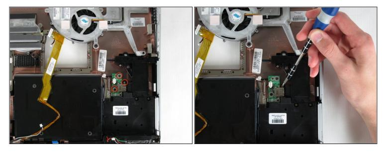
• Unscrew the two 4mm and one 2mm Phillips screws from the USB board.
