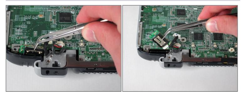
• Using tweezers, pull up on the Bluetooth module to remove it.
