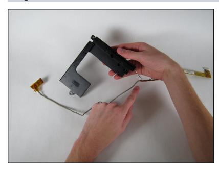
Cut the tape that attaches the USB cable to the left speaker cable.
