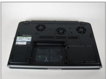
• Pull up on the battery to remove it.
