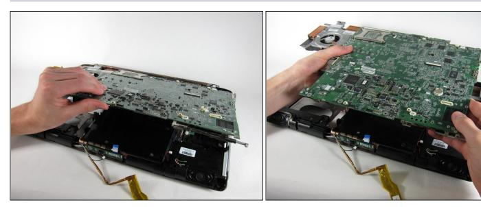
• Lift the motherboard up until it releases from the bottom casing and remove it from the laptop.
