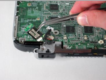
• Using tweezers, pull up on the Bluetooth module to remove it.
