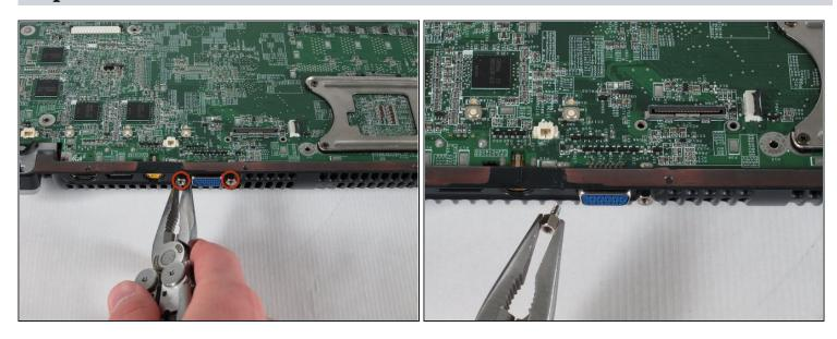
• Using pliers, unscrew and remove the two bolts from both sides of the blue VGA connector.
