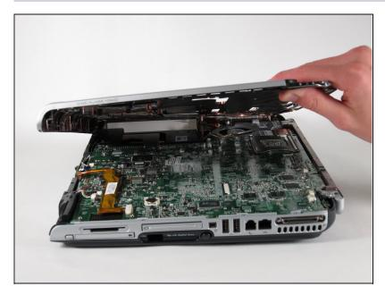
Lift the top cover from the left side to remove it completely.
