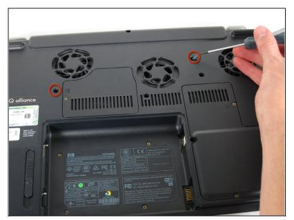
Remove the two 8mm Philips screws marked "K" on the bottom of the laptop.
