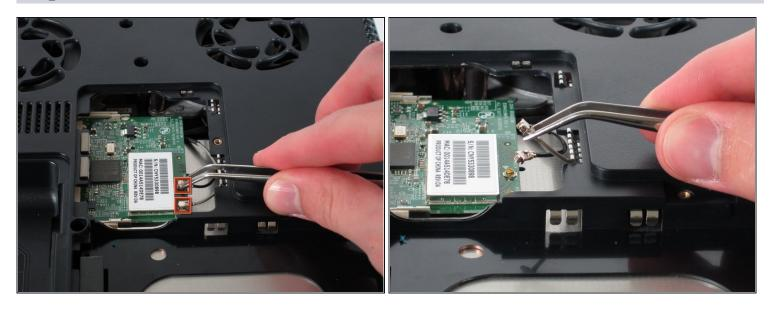
• Use tweezers to detach the grey and black cables connected to the green WiFi card.
