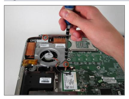
Unscrew and remove the two 8mm Philips screws from the heat sink fan.
