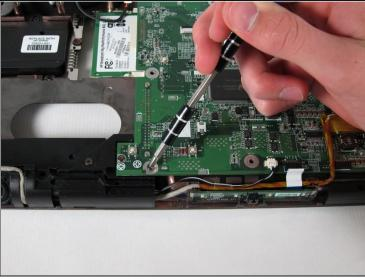
Unscrew and remove the five 4mm Philips screws marked with the white Phillips screw icon.
