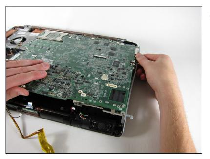
Pull the right casing to the side to release the ports on the motherboard from it.
