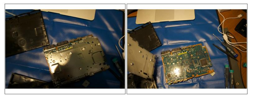
• Gently lift the metal casing from the motherboard. Place it to the side.
