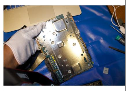
• Remove the single 2.4 mm screw located on the metal casing at the top of the motherboard.
