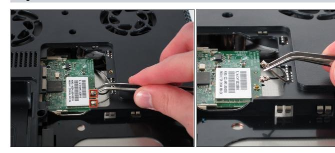
• Use tweezers to detach the grey and black cables connected to the green WiFi card.
