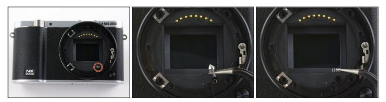
Use tweezers to lift the pyramid screw and spring from the lens assembly.
