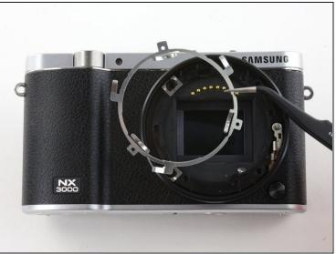
• Use tweezers to remove the black plastic ring and small metal ring inside the lens assembly.
