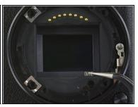
• Use tweezers to lift the pyramid screw and spring from the lens assembly.
