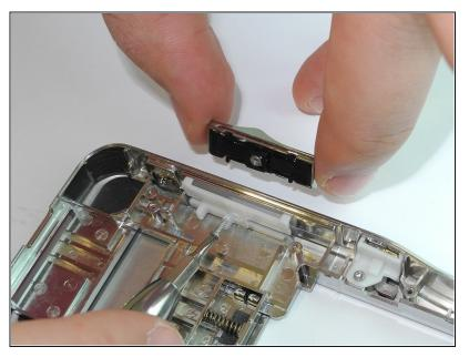
Remove the defective BA-Slider and replace it with the new one.
