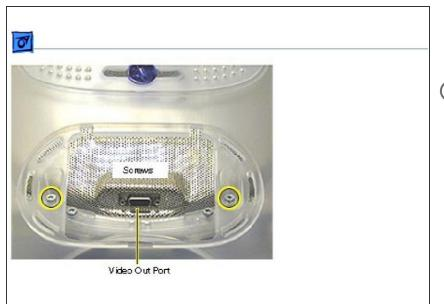
• Remove the two outer screws located near the video out port.
