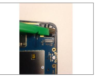
• Use a plastic opening tool to lift the rear facing camera connector off the pcb.
