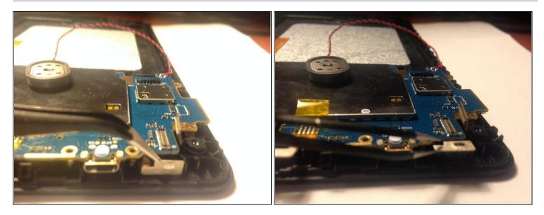
• Use heat and tweezers to lift the Power Button cable from the plastic frame.
