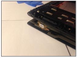
• The digitizer cable is threaded through a slit in the plastic frame. Unthread this cable carefully if you need to save your digitizer.
