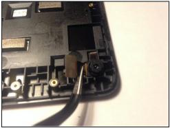
• Use tweezers to pull up the conductive tape from the frame, then lift the camera out of the frame.
